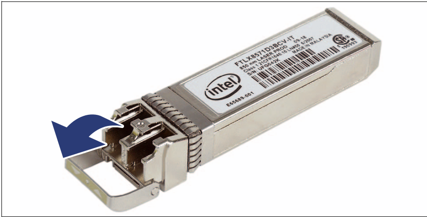
Figure 55: Unlatching the locking bail
